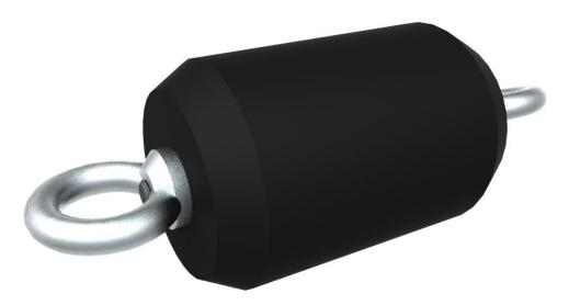
The Pipe Equipment Specialists Solid Proving Pig is used to prove that the internal dimensions of a pipe or duct, do not fall below a minimum diameter, and that the pipe/duct has a circular profile. The Solid Proving Pig is simply pulled through the pipe/duct.
