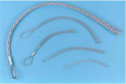
Towing Socks (Stockings), also known as Chinese Fingers, Pulling Stockings and Cable Grips can be used for any application that requires a pulling load to be applied to a cable, pipe, tube or similar object. These can be used either above or below ground, their most common use being for the installation of cables. They work on the principle 'the harder the pull, the tighter the grip'.
