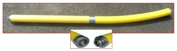
PECS (PE Coil to Straight) Connectors are a fully reusable product developed to overcome the problems encountered when passing coiled PE pipe through service cut outs whilst slip lining an existing metallic pipe using a pushing device attached to a mini digger.
