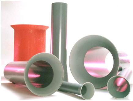
The Pipe Equipment range of Insertion Trumpets has been specially developed to eliminate the possibility of damage to PE pipes caused by the cut edge of the existing metal pipe during a dead insertion or slip lining operation.
