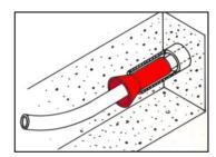
Once the PE is installed the Insertion Trumpet can be either removed or, for added security left in-situ to protect the PE from further damage from the metal pipe edge.
